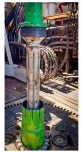
force of 270 mTon (595 klbs) to free the 7 inch x 95% inch dual cemented casing section.
